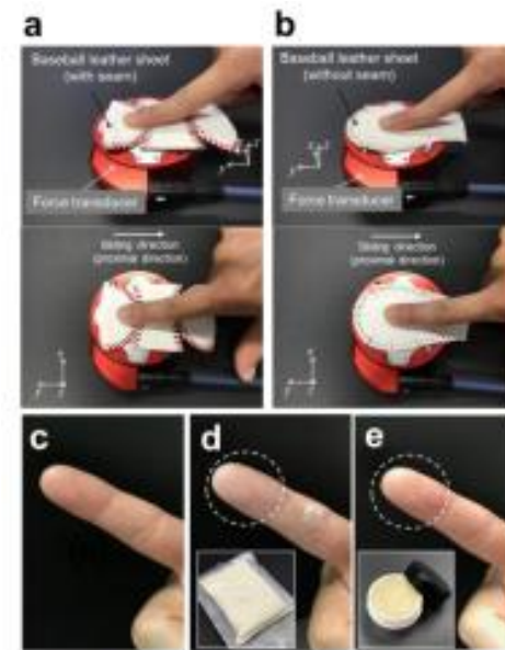
Fig. 1 Experimental setup for friction test between index finger pad and MLB ball leather sheet 1)
